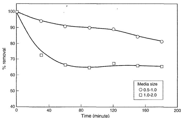
**Figure 8: The change of turbidity removal ratio with time for the pumice bed under the different grain sizes (15.28 m<sup>3</sup>/m<sup>2</sup>.h flow rate, 750 mm bed depth).**
