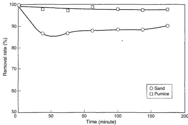
**Figure 10: The comparison of turbidity removal ratios with time for the pumice and sand bed (750 mm bed depth, 7.64 m<sup>3</sup>/m<sup>2</sup>.h flow rate & 0.5-1.0 mm grain size).**
