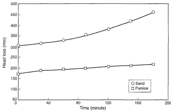
**Figure 9: The comparison of head loss values with time for the sand and pumice bed (750 mm bed depth, 7.64 m<sup>3</sup>/m<sup>2</sup>.h flow rate & 0.5-1.0 mm grain size).**
