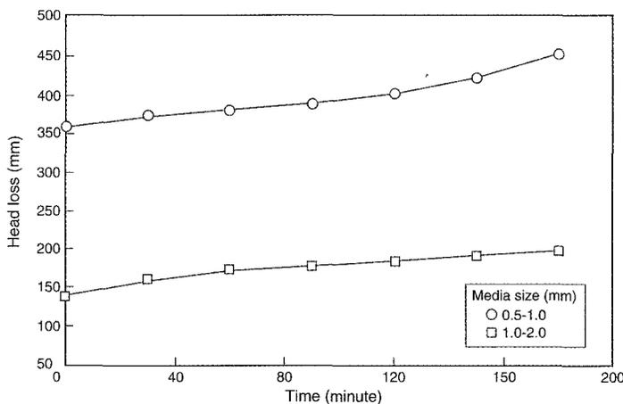
**Figure 7: The change of head loss values with time for pumice bed under the different grain sizes (15.28 m<sup>3</sup>/m<sup>2</sup>.h flow rate, 750 mm bed depth).**
