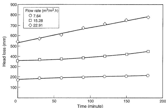
**Figure 3: The change of measured head loss values with time for the pumice bed under the various flow rates (750 mm bed depth, 0.5-1.0 mm grain size).**
