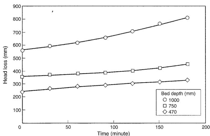
**Figure 5: The change of head loss values with time for the pumice bed under the various bed depths (15.28 m<sup>3</sup>/m<sup>2</sup>.h flow rate, 0.5-1.0 mm grain size).**
